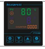
Press the power switch to turn on the machine, then press the "SET" button
