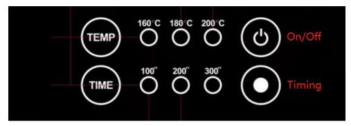
A: Press TEMP button to set the temperature. B: Press TIME button to set the time.
